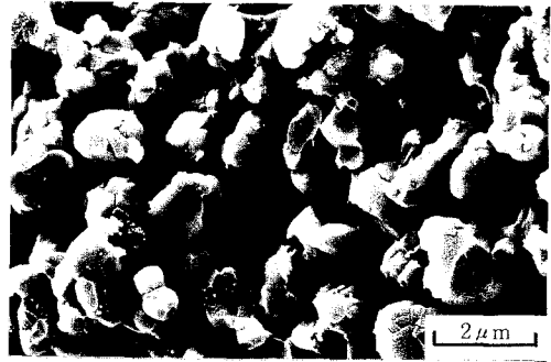
Fig. 1. SEM micrograph of the fractured (Ba,Sr)TiO 3 surface.
