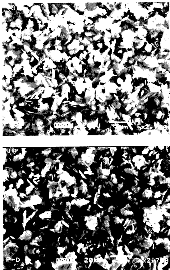
Fig. 2. Secondary electron images of precursor powders (a) P-1 and (b) P-2.
