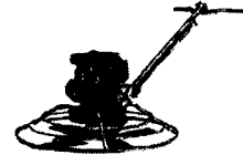
Fig. 1 Conventional concrete floor finisher
