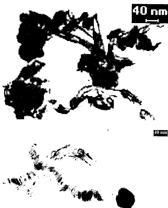
Fig.5. Electron-microscopic photograph of over-carbonized chrome sludge at T = 800\text{ }^{\circ}\text{C} .
