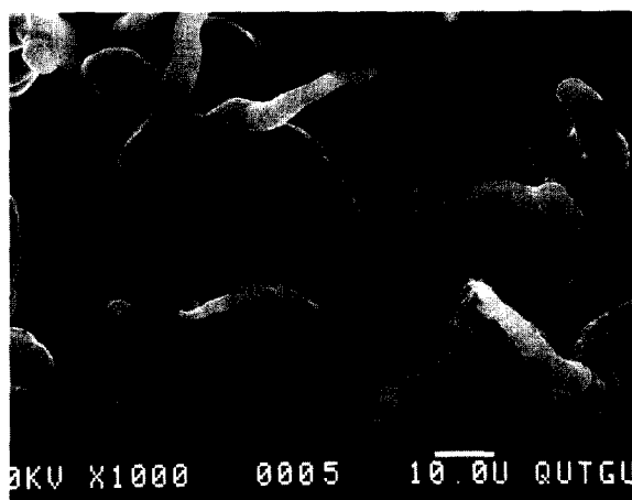
Figure 5. SEM micrograph of a highly pTS doped (0.05 M/l p-TS) film synthesized at room temperature for 1 hour. Magnification 1000X.
