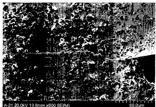
Fig. 1. Crack propagation of Al 2 O 3 -dispersed Y-TZP ceramics.
