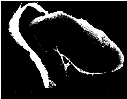
Fig. 16. Scanning electron micrograph of the cross section of fiber beaten for 30 min.
