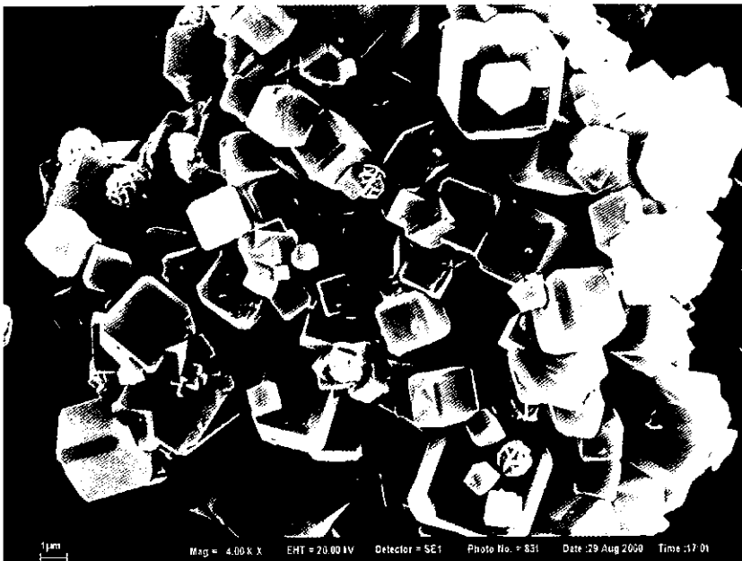
Fig. 3. Scanning electron micrograph of zeolite cubo-dodecahedral Na-A synthesized from funnel-glass waste. T=80°C; reaction time=3 hours.
