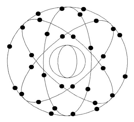
FIGURE 1. Schematic picture of the GPS constellation: 6 planes with at least 4 satellites in each. Each satellite is about 15 minutes less than 2 orbits/day.
