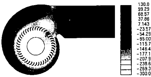
Fig. 5 Static pressure contours on a mid-span plane.
