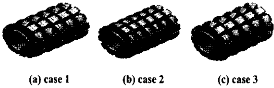
Fig. 15 3-dimensional geometry of gerotor hob by changing eccentricity and arc radius
