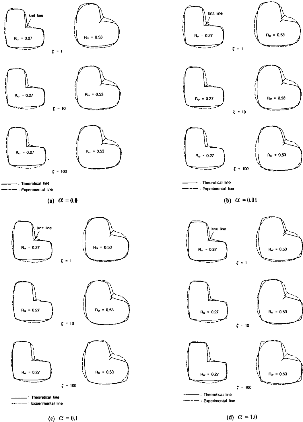
Fig. 5 Comparison between theoretical and experimental results for flow fronts
