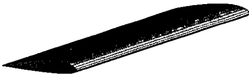
Fig. 4 Patch distribution on NACA3317 airfoil
