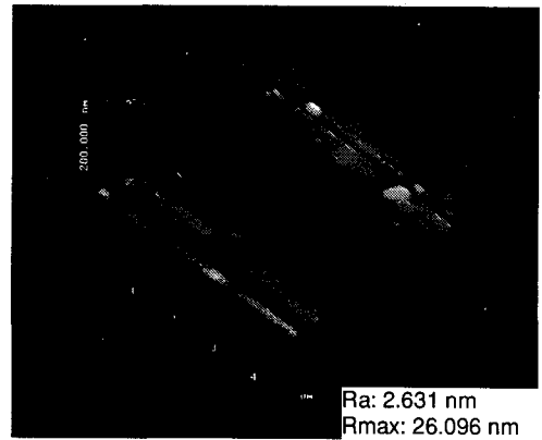
Photo. 1 AFM image of silicon nitride ground by a #4000 CIB-D wheel
