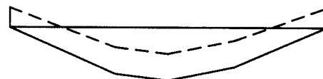
Moment Diagram without Moment at Supports ——— Moment Diagram with Moment at Supports - - -
