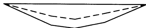
Stress Diagram by Non-Composite Section Modulus ——— Stress Diagram by Composite Section Modulus - - -
