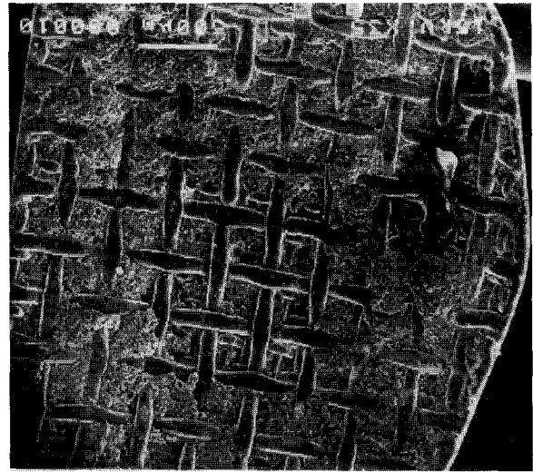
Fig. 5. SEM image of the bracket base after debonding (Group 4, AP-GI, magnification \times 35 ) (surface treatment : acidic primer, adhesive : Fuji Ortho LC ® , mean value of ARI : 2.1)
