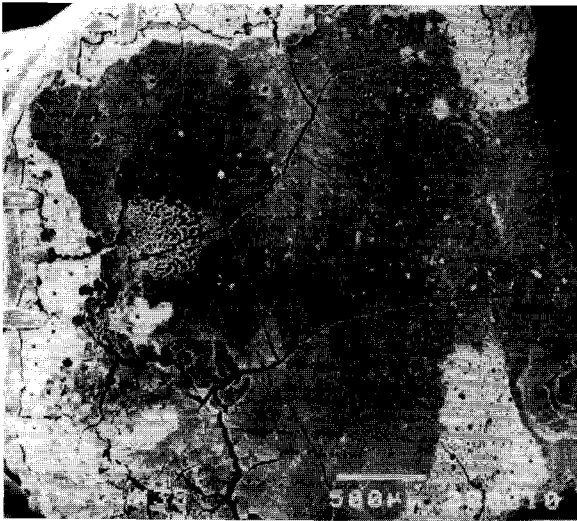
Fig. 4. SEM image of the bracket base after debonding (Group 3, AP-P, magnification \times 35 ) (surface treatment : acidic primer, adhesive : Panavia 21 ® , mean value of ARI : 0.2)
