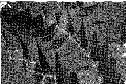
Fig. 7 Velocity distributions at midspan
