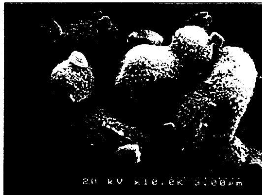
Fig. 6. Scanning electron micrograph of the perovskite-type catalyst doped on Al 2 O 3 support(Magnification value 10,000×).
