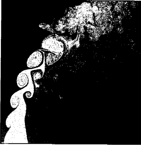
Fig. 2 Instantaneous tomographic image at the centerplane, Re_D = 1050
