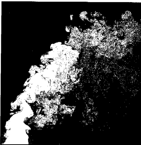
Fig. 3 Instantaneous tomographic image at the centerplane, Re_D = 2100
