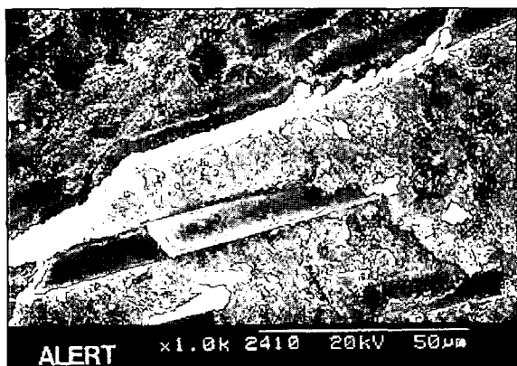
Fig. 5. Scanning electron microscope shows fractured surface of ALERT. Dislocation of rod-shaped fillers from resin matrix and fracture of rod-shaped filler were observed( \times 1000 ).
