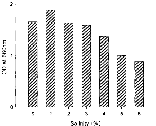
Fig. 6. Effect of NaCl on the growth of Enterobacter sp. CW-6 in nutrient broth after 48 hours culture at 35°C.
