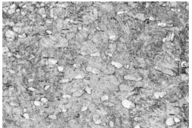
Photo 6-2. Microstructure of bronze bowl II( \times 100 ).
