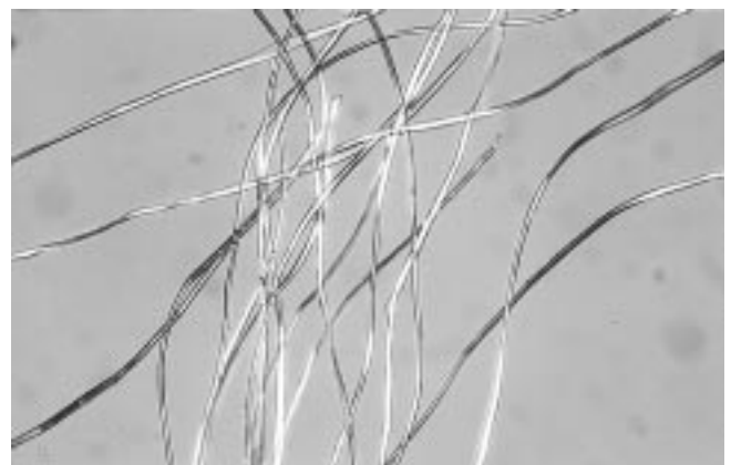
Photo 3-3. Silk fiber, the quilted jangyee under SEM(X100), diameter of fiber : 8-10 \mu\text{m} .
