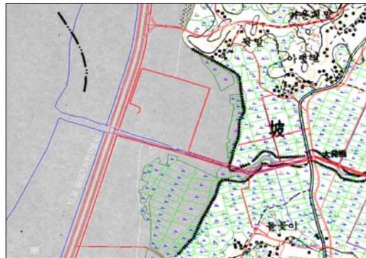
FIGURE 13. Update of an existing map by overlaying the newly produced digital map
