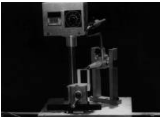
Figure 1. Sledge device used for instrumentation. Lateral force and instrumentation time can be adjusted.
