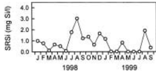
Fig. 5. Monthly variation of soluble reactive silicon (SRSi) concentration in the Kum River-Reservoir from January 1998 to September 1999.
