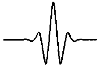
Fig. 3 The Mother wavelet used in the wavelet analysis(bior2.8), which is similar to the actual ultrasonic pulse
