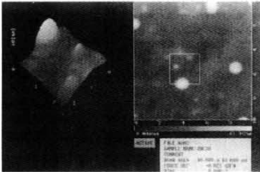
Figure 7. AFM image of the polyimide/silica hybrid composite film with 30 wt% TEOS loading. [27]
