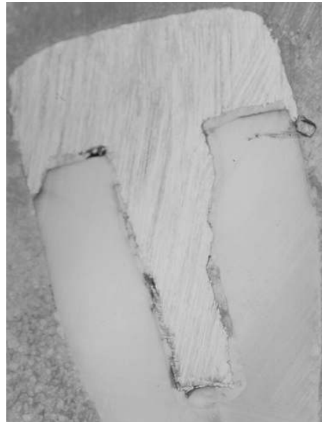
Fig. 3. Microleakage of Group (Fleck's)
