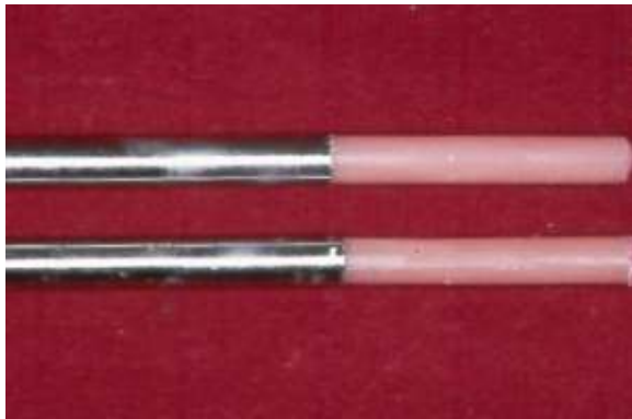
Fig. 5. Complete metal-relining material specimens before tensile testing.
