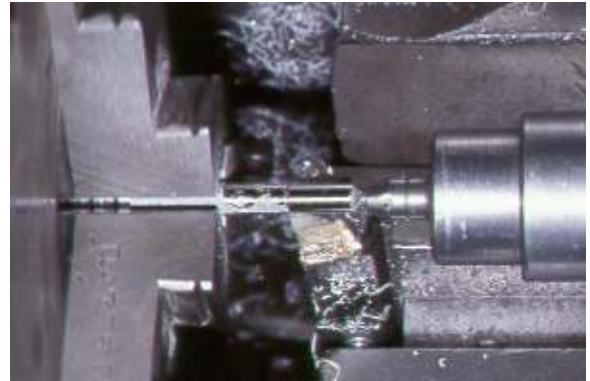
Fig. 2. Specimens undergoing milling procedure for 6.0mm diameter.
