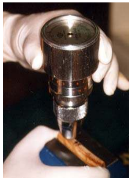
Figure 9. The measurement of removable torque with torque gauge(Kanon Mfg. Co. Japan)
