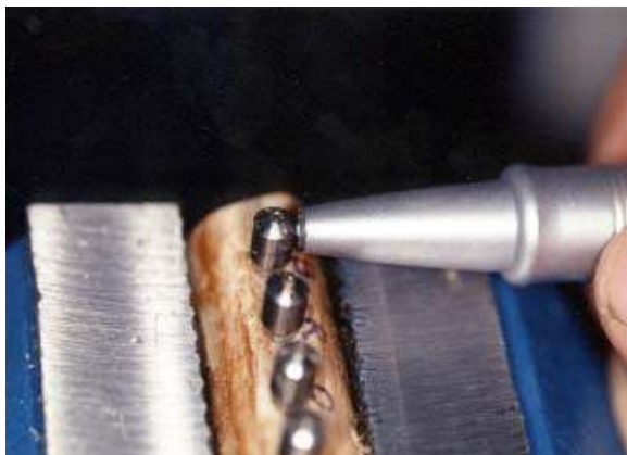
Figure 8. The measurement with Periotest ®
