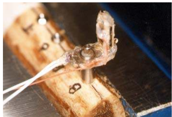
Figure 7. The measurement RFA transducer connected with implant.
