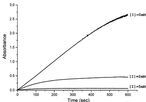
**Figure 2.** To determine the efficiency of enzyme inactivation by salioxon, we continuously monitored at 405 nm and 25 °C by a JASCO UV/Vis spectrophotometer equipped with a JASCO peltier type thermostatic cell holder (method C).
