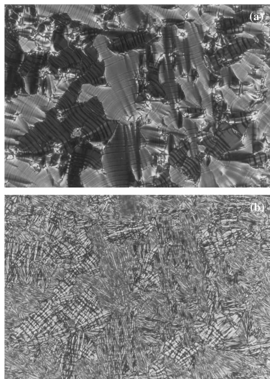
Figure 8. Photomicrographs of compound 10 with x = 8 on cooling (magnification of \times 250 ): (a) 235 °C; (b) 177 °C.
