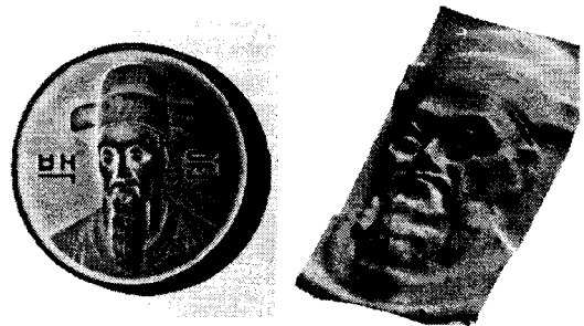
Fig. 10 Measurement result by shadow moire
