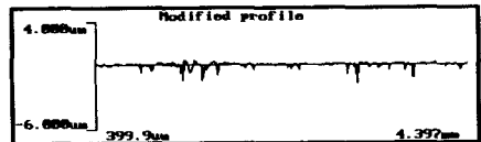
Fig. 23 Modified profile of electrochemical grinding( R_{max} 2.145\mu m )
