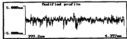
Fig. 21 Modified profile before machining( R_{max} 5.752\mu m )
