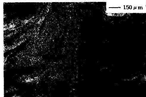
Fig. 8 Microstructure of C-4 after potentiodynamic test at 0.11M H_2SO_4
