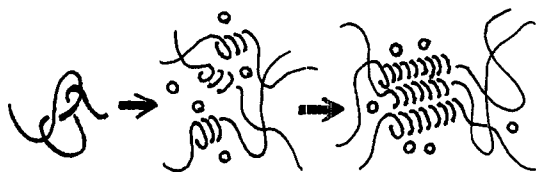
Figure 11. An illustration of solvent-induced structural ordering process of sPS glass sample.
