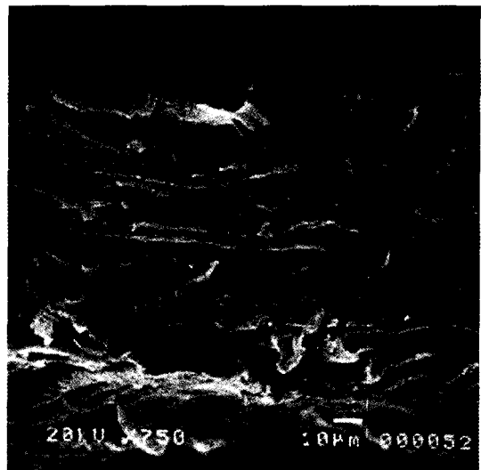
Fig. 10(d). SEM photograph after soft nip calendering. Heating roll temperature: 160°C, Pressure: 207 kg/cm 2 .
