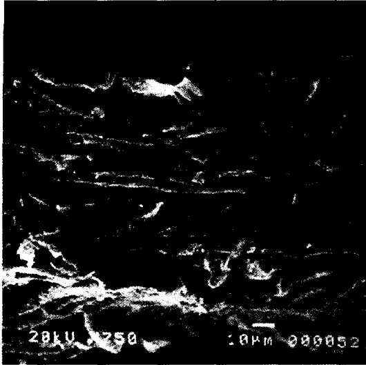
Fig. 10(a). SEM photograph of uncalendered sheet.
