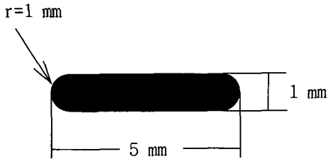
Fig. 4. Shape of sensor core (thickness of 25 μm).
