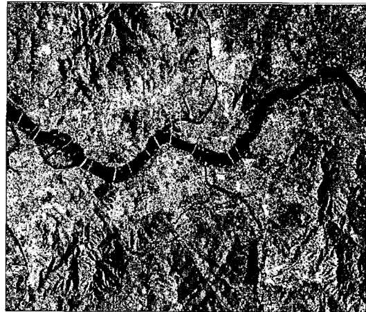
Fig. 15. SAR Image Processed for Standard Mode with 10m Resolution Around Han River in Seoul
