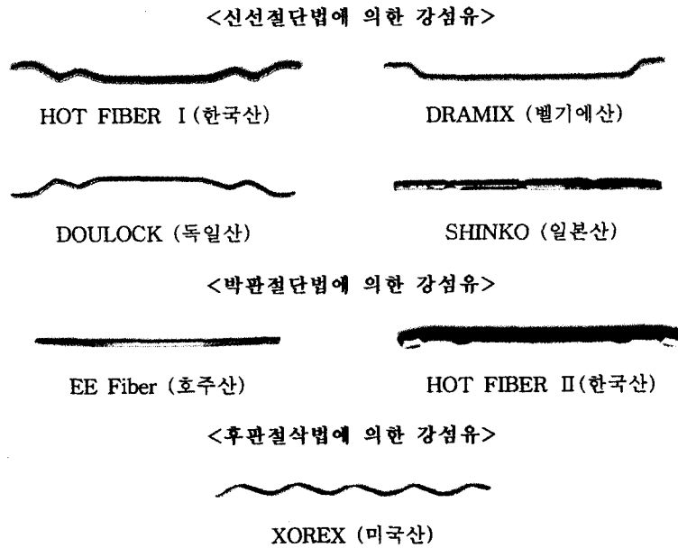
Fig. 1. Classification of steel fiber currently being used in Korea
