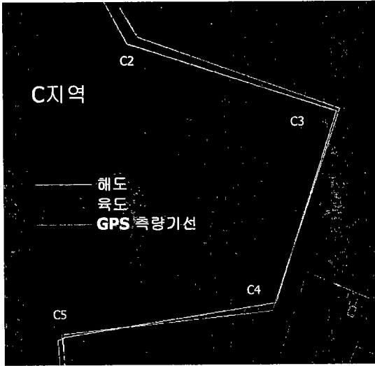
Fig. 5 Overlay of GPS Survey Data and an Integrated Digital Map
