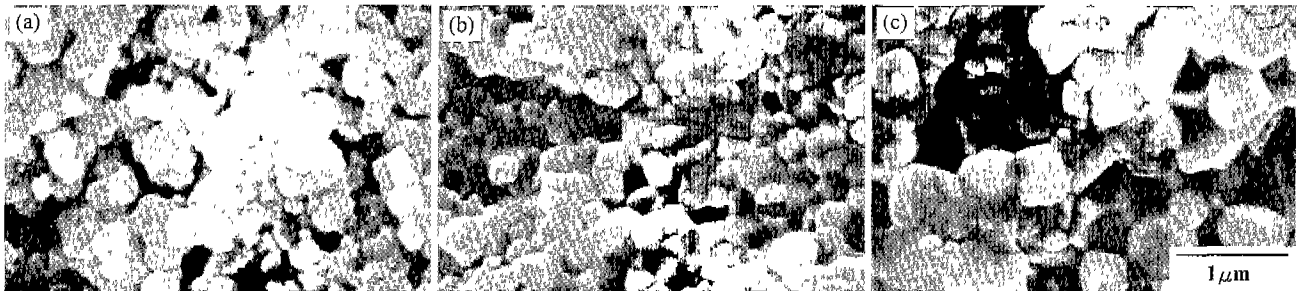
Fig. 10. SEM micrographs of fracture surface after bending test in zirconia prepared by pressureless sintering; (a) 1300°C, (b)1400°C and (c)1500°C.
