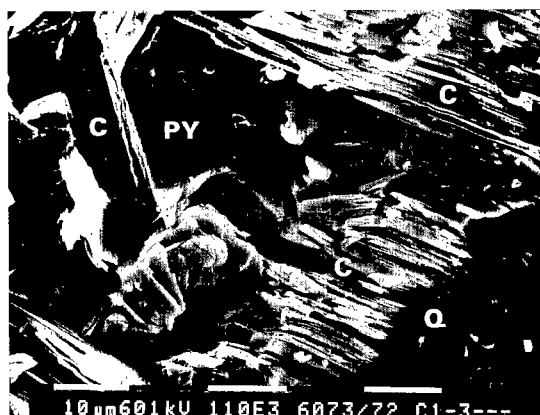
Fig. 3. Scanning electron micrographs of chlorite in sample C1-3 showing well-crystallized chlorite (C) around pyrite (PY) and quartz (Q).
