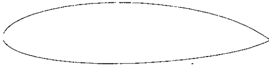
Fig.1 Shape of 2-D Hydrofoil (KH55)
