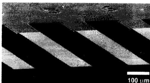
Fig. 18 Scanning electron micrograph of a section of a microfabricated silicon cantilever array (eight cantilevers, each 1  $\mu\text{m}$  thick, 500  $\mu\text{m}$  long, and 100  $\mu\text{m}$  wide, with a pitch of 250  $\mu\text{m}$ , spring constant 0.02 N/m; Micro and Nanomechanics group, IBM Zurich Research Laboratory, Switzerland) (from<sup>[31]</sup>).
