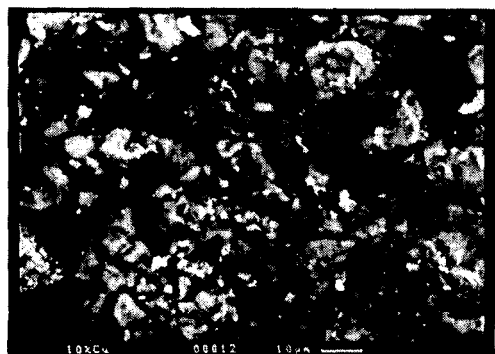
Fig. 2. SEM-BEI micrographs of samples ; 5wt% Cu/Al 2 O 3 (a), 10wt% Cu/Al 2 O 3 (b). white spots show copper location.
