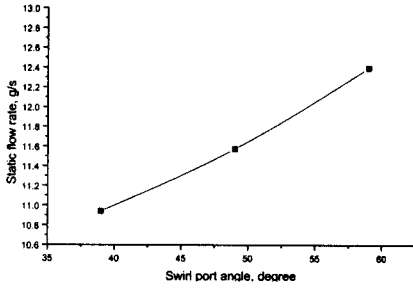
Fig. 14 Variations of the static flow rate as a function of the swirl port angle
