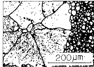
(a) Large and small grains in duplex structure after the sintering for 20min
