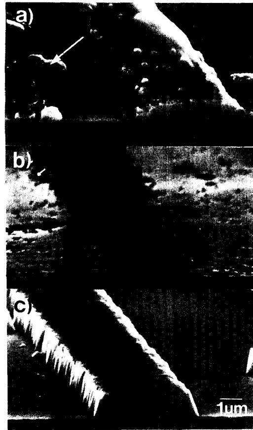
Fig. 3. Cross-sectional SEM micrographs of a mesa etched at 800W-5mTorr-60%BCl 3 -10min. The bias voltage is (a) 200V, (b) 100V, and (c) 300V. The arrow indicated the surface residues.
